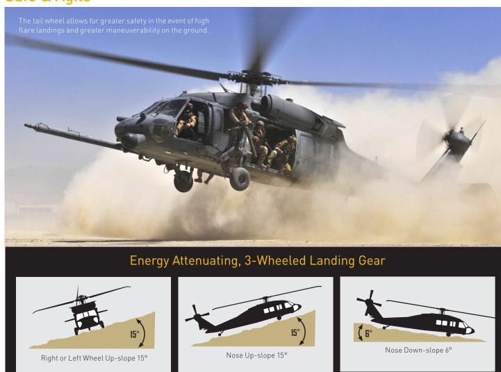
Energy attenuating, non-tricycle, wheeled landing gear designed for unprepared landing zones and sloped areas:
